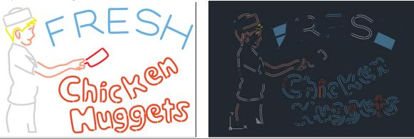
You can still include color in the drawing if it is only the lines that are colored. Figure 3 shows an example of a PDF file that has all the appropriate linework and imports well into AutoCAD (Figure 4.)
